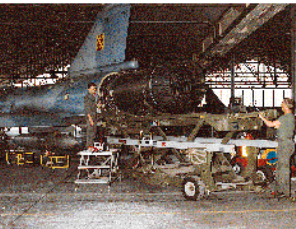
M53 engine removal.
