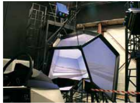
The cockpit is equipped with a high resolution/wide field display in a pseudo-sphere composed of 8 back-screen projected facets. It includes real equipment and can be reconfigured for forward and rear seats to simulate a two-seater by coupling two single-seater cockpits. It is also equipped with a Sogitec G-seat inclined at 30°.
