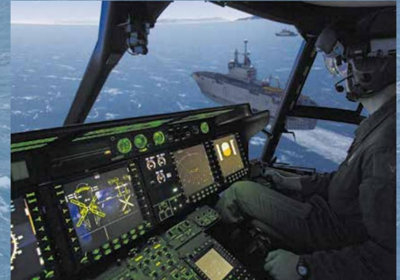
Sogitec NH90-NFH simulator cockpit with Sogitec Apogée™ 7 latest image generation system and very high definition spherical screen.
